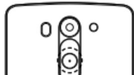
Press and hold the **Power/Lock** key for a couple of seconds.
